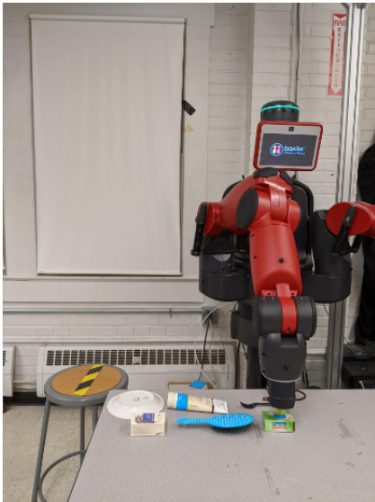
Fig. 6: An example of Baxter robot cleaning objects belonging to class soap from a set of objects in front of it's arm camera on the table.
