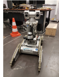
Fig. 1: Tracked robot equipped with a RGBD camera
