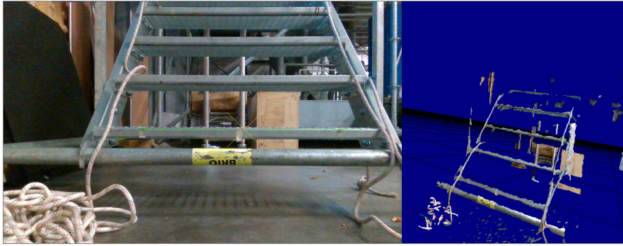
Fig. 7: Industrial stair data from the RGBD camera The thin green line corresponds to the located stair in the RGB image
