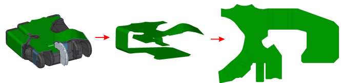
Fig. 3. From 3D shape to flat shape contour to be used as a guide for developing the flexible PCB, the base of the palm sensor. (left) The 3D model of the sensor shape is constructed in CAD to cover the palm. (middle) The sensor shape in 3D without SDRH. (right) Flattened shape of the sensor. (For simplicity, middle and right images do not show the little finger metacarpal unit)
