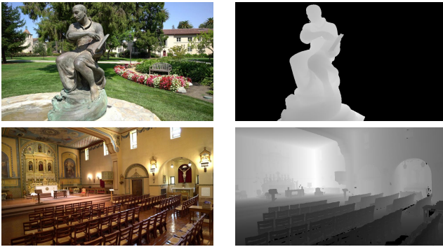
Fig. 1. Frames (left) and ground truth depth maps (right) from the Ignatius and Church scenes
