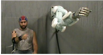
(a) Experiment I : The subject moves their hand in 3D space, tracking it with their eyes. The robot replicates the motion.
