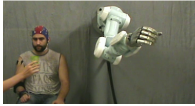
(b) Experiment II : The subject follows a moving object in 3D space. The robotic arm follows the trajectory of the object.
