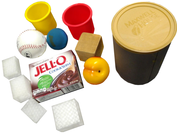
Fig. 5. Set of objects that were used in the grasping experiments. The dimensions of the everyday objects used can be found in [24]. The 3D printed objects have the following dimensions: 10x35x50 mm, 22x35x50 mm, 32x35x50 mm, and 50x35x50 mm.
