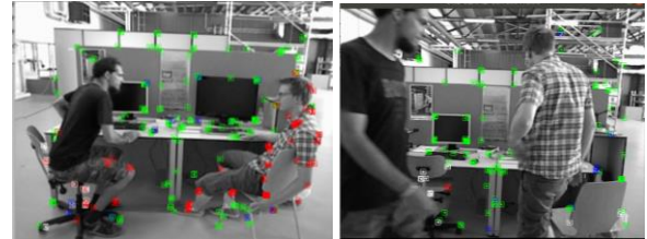
Figure 1. Static feature points extracted from movable objects are shown in red and white points represent feature points extracted from static but movable objects like chairs. Green points and blue points represent feature points extracted from static objects which have appeared several times and only one time respectively.
